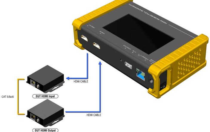
Procedure of Loop Test: \*only support 1080p@60, 4K2K 30Hz and 4K2K 60Hz resolution
