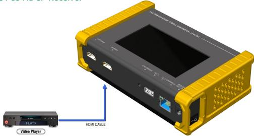
When AV-GM0923-S1 set as receiver, it can verify HDCP of video player or other DUT (Device Under Test). AV-GM0923-S1 provides three options (HDCP 1.4 / HDCP 2.2 / no HDCP) for users to select and confirm the HDCP authentication of DUT.
