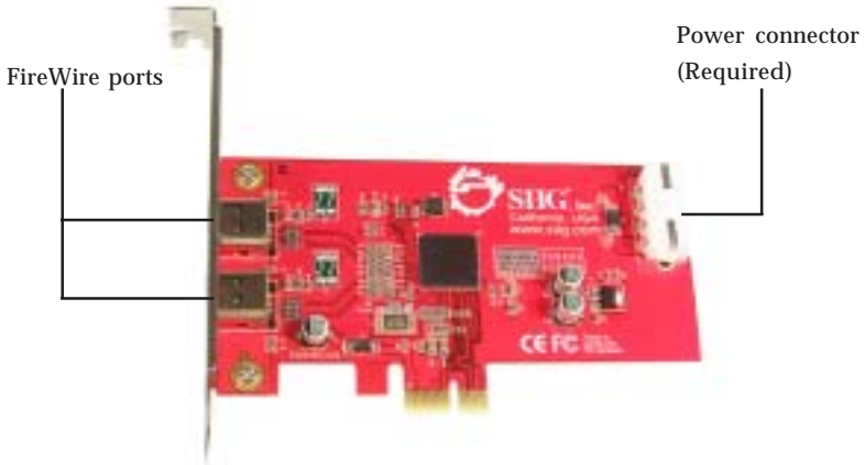
Figure 1: FireWire 2-Port PCIe DV Board Layout
