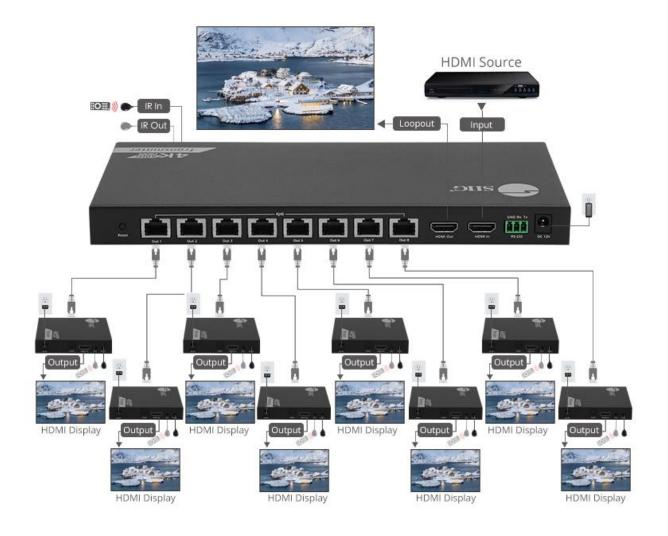
With the ability to extend HDMI signals up to 230ft (70m) via Cat6/7 cables, these extenders are perfect for large spaces like auditoriums or exhibition halls. Additionally, their near-zero latency ensures real-time performance, crucial for applications like video conferencing and live broadcasts.
