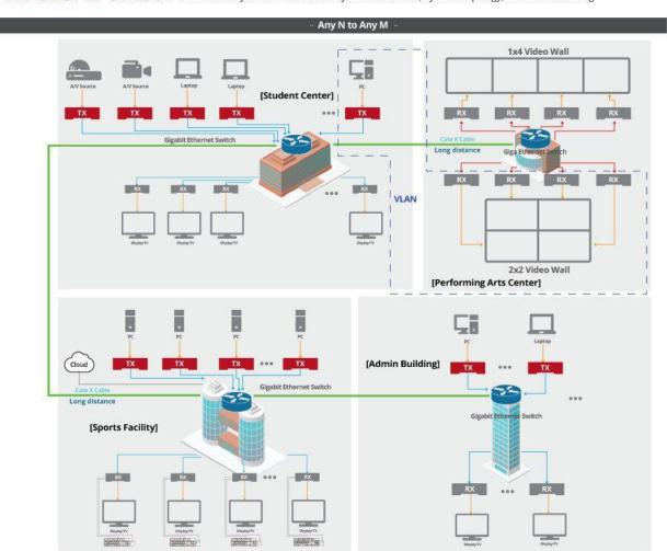
AV over IP Solution - Showcase any number N of TX to Any number M of RX, dynamic topology, shared CATx cabling
